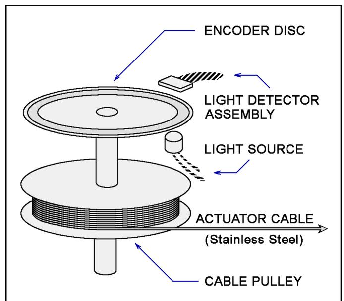
*Simplified diagram of encoder operation.*
