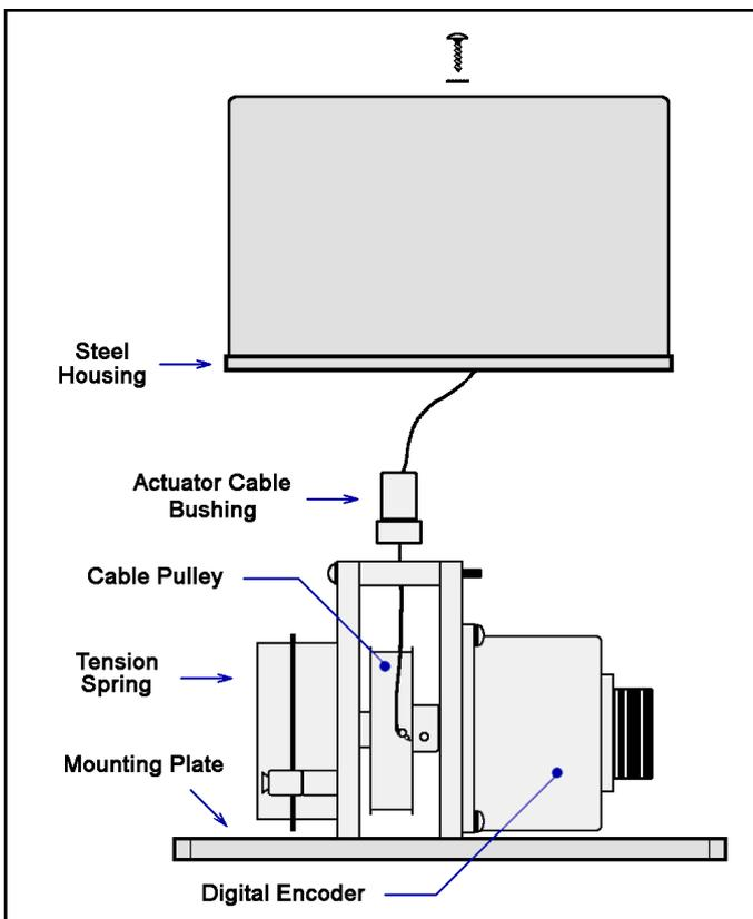
*Cable-actuated digital position encoder.*
