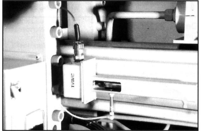
*Digital encoder assembly with cable guard.*
